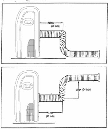
**Incorrect hose mounting** (Air exhaust bend is too large and can cause a malfunction).
